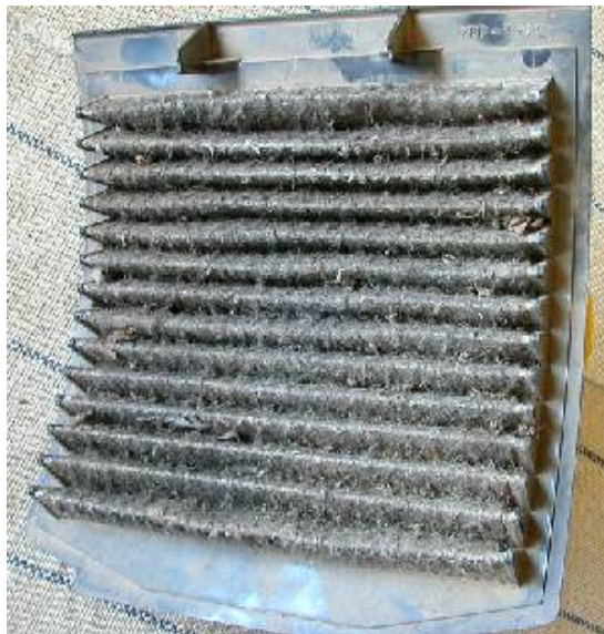
Fig. 5: Pollen car filter eliminating dust and other particles from incoming air
