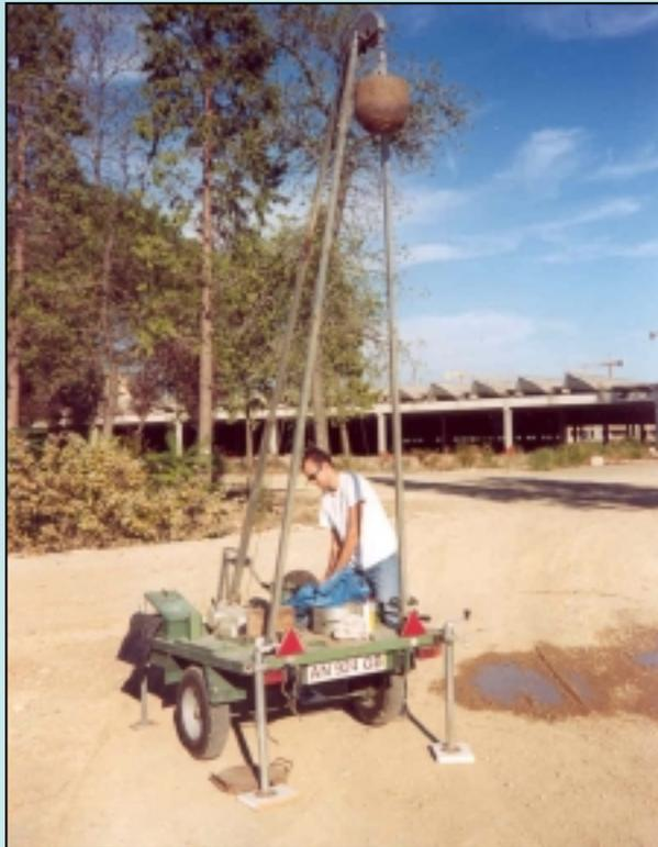
Dropped weight as a seismic source
